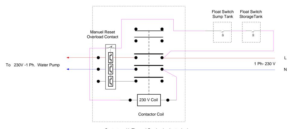
Contactor with Thermal Overload unit attached
