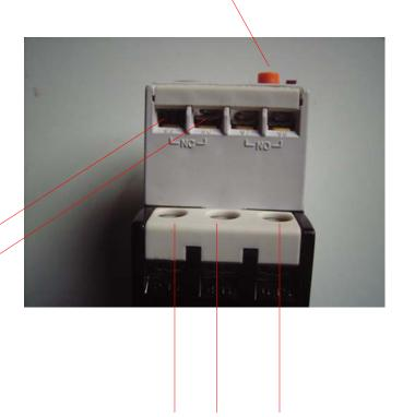
T1, T2 and T3 terminals of the Thermal Overload unit
